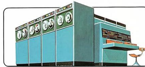
▲ The first electronic computer went into operation in 1943. Using bulky valves in its circuits it sprawled across 160 square metres. In the 1950s small transistors replaced valves and a modern computer like the one above takes up only a few metres. The latest computers have transistors in 'micro-chip' form reducing the size of their electronic 'brains' thousands of times. Computers are good at arithmetic, but they cannot (as yet) think for themselves.
