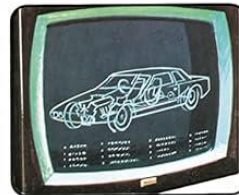
▲ This picture shows a computer at work in the car industry. Designers have the car's shape displayed on a TV screen. The image can be viewed from any angle and changed easily until the body style is decided upon, making designing quicker and cheaper.
